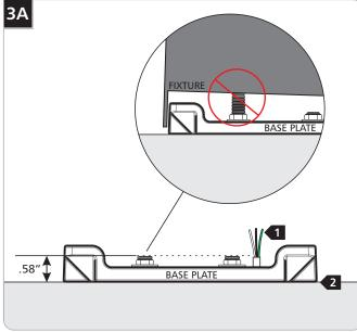
**Warning:** the mounting plate placement is off-center in relation to the center of the fixture on some models. Make sure to place the fixture in the desired location and determine the correct mounting plate placement before installing the mounting plate.
