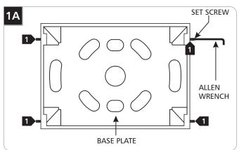
Loosen (**Do Not Remove**) the four set screws on fixture base with the provided Allen wrench and remove the base plate.
