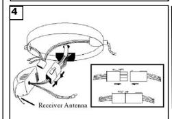
Connect the molex from the receiver to the molex in the switch housing plate by aligning and sliding together. Note: For longer distance operation, coil receiver antenna around the natural wire (white wire).
