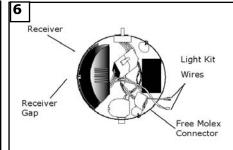
Align gap in receiver with the screw between speed switch and reverse switch and slide receiver (Dip switch facing housing plate) into switch housing plate. Receiver should fit directly into area in the switch housing plate. Note: If installing light kit, use the blue and white wire from the receiver.
