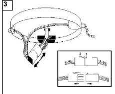
Disconnect Molex Connectors in switch housing plate by pushing down on tab and pulling the two (molex connectors) apart.
