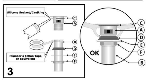
\* Approved sealant alternatives may be used to ccommodate for installation requirement.
