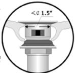
Install the pop-up exactly using the instructions below. Use a bead of silicone sealant around the C, upper gasket, to avoid any possible leaks.
