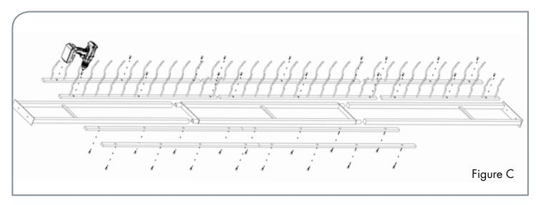
**3. Assemble the frame** - Slide the frames together. Secure the W Series racking and/or FCF Backer Bars to the front and back of the frames using provided self-drilling screws (Figure C). Ensure the connection joints of the frames are supported by either W Series wine racks or an FCF Backer Bar. The connections must be supported by a minimum of 12" of racking or backer bars (Figure D).
