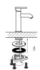
4. PLACE NEW FAUCET IN THE POSITION ON THE SINK. FROM UNDER THE SINK, PUT GASKET AND METAL PLATE AND THREAD NUT ONTO THE PIN. TIGHTEN THE NUT. PLACE SET SCREWS IN TO THE NUT AND TIGHTEN THEM.
