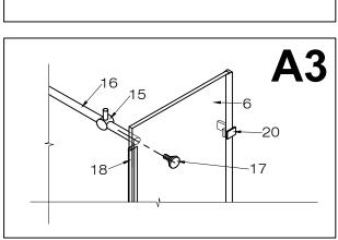
4. Place the side glass panel (#6) with the structural rail (#16) into desired position. Use the level to correct position assembly. Mark holes on the wall for the side glass support (#20). Mark the circumference location for the wall mount bracket (#1). NOTE: Make sure to keep the side glass panel perpendicular to the structural rail. Failure to do this can lead to the glass breaking and bodily harm.
