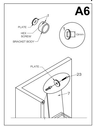
7. Place the side glass panel and the structural rail back to the shower opening. Screw the side glass supports to the wall with 1 5/8" screws (#22). There is a 10mm adjustment built into the glass supports for minor modifications. Thread the wall mount bracket body (#1) back onto the plate and tighten the set screw using the hex key supplied. Tighten the structural rail screw (#17).
