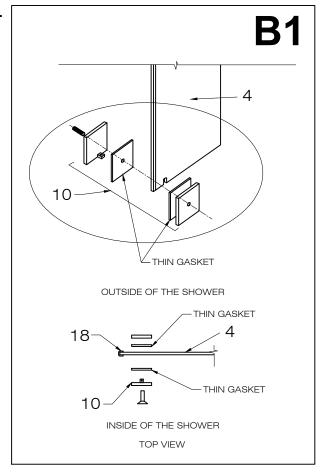
2. Place the side seal strip (#18) on the big front fixed panel (#4) on the side of the wall.
