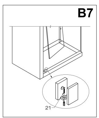
8. Align the big front fixed panel to the shower opening location. Screw the big front fixed panel to the structural rail with the fixed panel holders. Screw the fixed panel bottom clip (#10) to the big front fixed panel.
