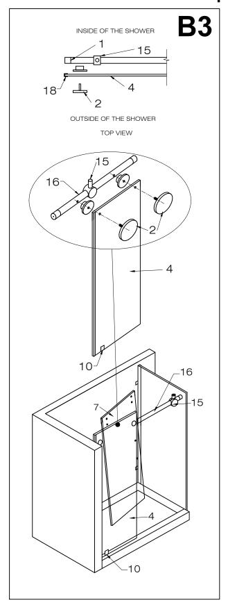
Make sure the front fixed panel is level and mark the fixed panel bottom clip (#10) location on the floor.
