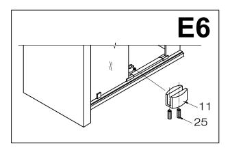
7. Screw the door guide to the floor with 1 1/8" screws (#21).
