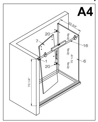
5. Remove the side glass panel (#6) and the structural rail (#16). Drill holes into the wall where marked for the glass supports (#20) and in the center of the circumference of the wall mount bracket (#1) \*70 1/4" and place plastic anchors (#24) in them.
