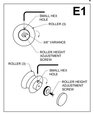
Use the provided allen key to unscrew the adjustment screw and dismantle the roller. Place the screw through door panel top holes and attach the two top rollers onto the door panel (#7).
