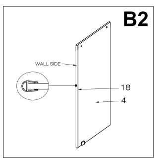
3. Place the big front fixed panel (#4) in the shower opening making sure to have the fixed panel bottom clip (#10) closer to the wall. Screw the big front fixed panel to the structural rail (#16) with the fixed panel holders (#2).
