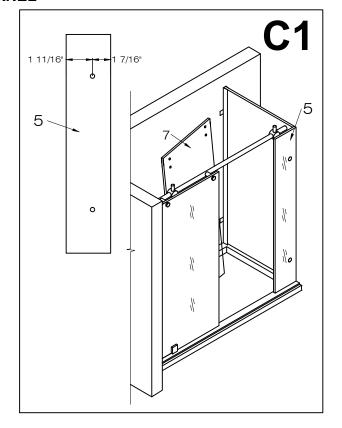
2. Unscrew the corner brackets (#8). Align the corner brackets to their respective positions from inside the shower. Place the corner plates on the outside of the shower. Screw in the corner plates to the corner brackets with the provided screw from inside the shower. The side seal strip (#18) will be firmly compressed between the small front fixed panel (#5) and the side glass panel (#6). This is to prevent water leakage.
