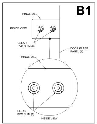
2. Place gaskets on each side of the door glass panel. Screw the hinges to the door glass panel with the hex key (supplied).
