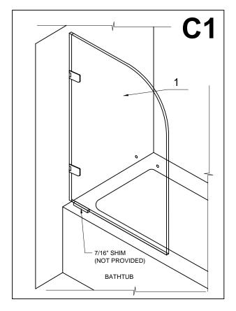
2. Align the door correctly using a level. Mark two (2) holes on the wall for the mounting screws for each hinge.
