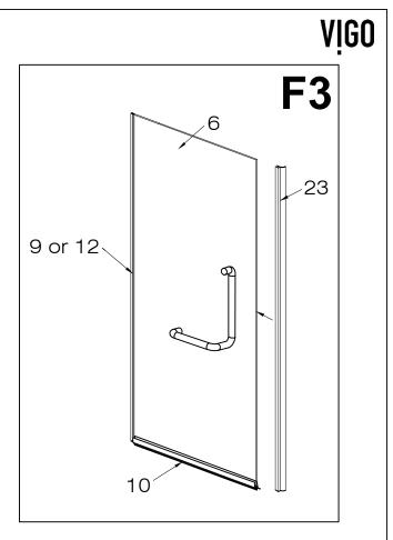
3. Install Door side seal strip (#23) the door panel.
