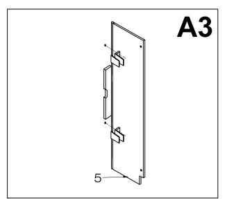
4. Remove the front fixed panel and drill holes into the wall. Insert plastic anchors (#17) into the holes. Not necessary if installing into studs. Studs are the preferred means of installation, anchors can pull out of the wall causing property damage and bodily harm. There is a 10mm adjustment built into the glass supports for minor modifications.
