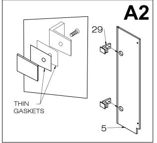
3. Mark holes on the wall for the mounting screws after leveling panel.
