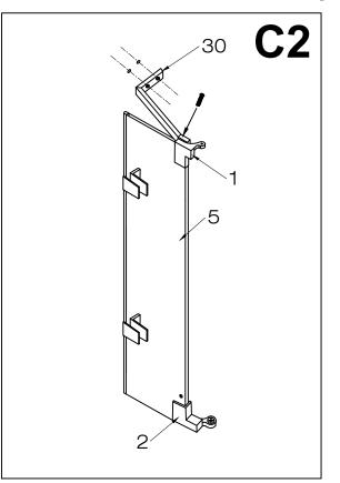
3. Remove the structural arm (#30) from the top turning hinge base and drill holes into the wall at the marked locations. Insert plastic anchors (#16) into the holes.
