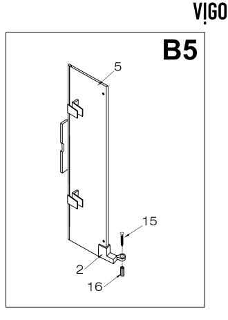
Remove the screw that connects the structural arm on the floor mount portion of part (#2). Removing this is to prevent personal injury, silicone the void to prevent water entry.
