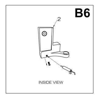
turning hinge base (#1). Note that the structural arm has an adjustable screw hole of 1/2" length. This will allow for flexibility and proper install placement.
