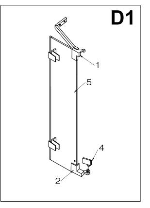
One installer manually inserts the convex portion of the turning hinge (#3) into the concave portion of the turning hinge base (#1) and holds the position. The hinges should be turned to a slightly open position.
