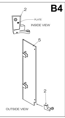
Screw the turning hinge base mirrored into the floor with 1 1/8" Phillips screw (#15). Make sure the glass panel is perpendicular to the wall.
