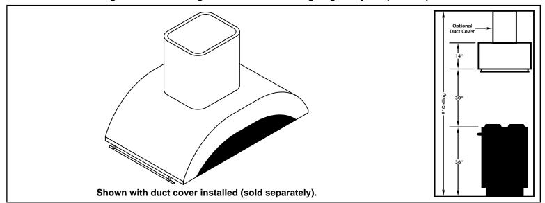
3) Load-bearing framework in the ceiling is necessary for the installation of an island hood. Additional framework construction may be required. Do not attach an island hood to a structure that cannot support twice the weight of the hood.
