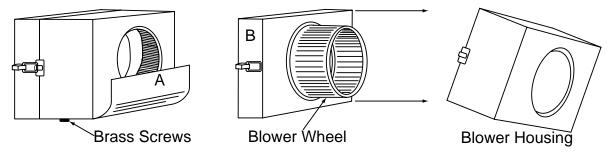
7) Remove the three screws retaining the blower motor(s). Unplug and remove the motor(s), taking care not to damage the blower wheel(s). It is not necessary to remove the blower wheel from the motor.
