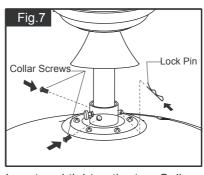
Insert and tighten the two Collar Screws. Slide Lock Pin into Hanger Pin until it locks into position.
