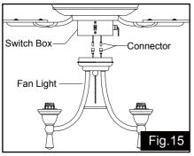
Make wire connections using the connectors respectivly from the switch box and fan light.
