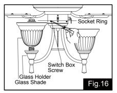
Secure the switch box with the switch box screws.
