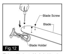
Tighten blades to blade holders by using blade screws.
