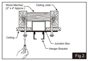
Tighten the hanger bracket to the outlet box with two mounting screws. (Make sure the outlet box is securely installed so that it will be able to support at least the fan weight.)
