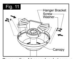
Remove the 4 hanger bracket screws and washers from the hanger bracket. Attach the canopy to the hanger bracket, then secure it with four screws and washers.
