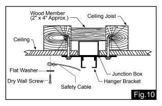
Attach the loop at the end of the safety cable to the ceiling surface, then secure it with a flat washer and dry wall screw. Make sure the flat washer and dry wall screw are covered by the fan canopy.
