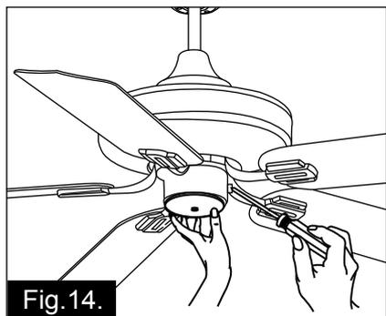
Step 14: Secure the switch box cover upward to the switch box with the switch box screws.
