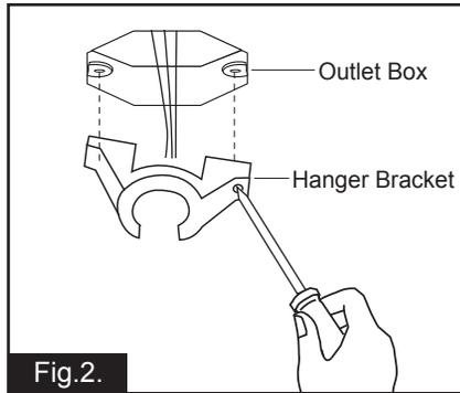
Step 2: Tighten the hanger bracket to the outlet box with 2 mounting screws. (To reduce the risk of fire electric shock, or personal injury, mount to the outlet box marked "Acceptable for fan support" and use mounting screws provided with the outlet box.)
