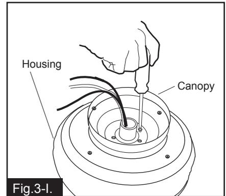
Step 3-I (for ceiling mount only): Attach the canopy to the housing with three ceiling mount screws.
