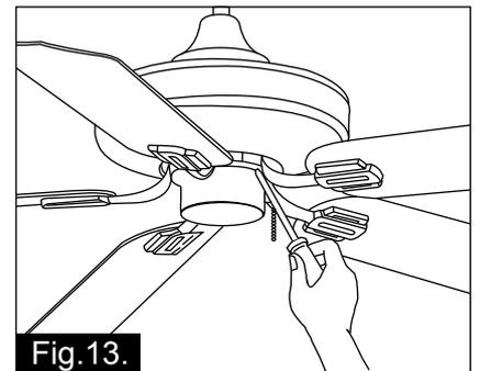
Step 13: Secure blade holders to the motor with motor screws and washers.
