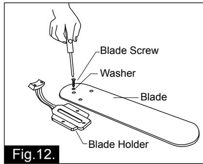
Step 12: Tighten blades to blade holders by using blade screws and washers.
