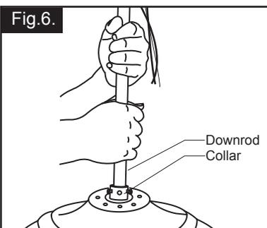
Step 6: Take off the downrod pin from downrod. Then insert the downrod into the collar.
