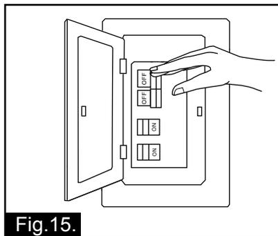
Step 15: Turn on the electric power at the main fuse or circuit breaker box. Use pull chain to control the fan speed.
