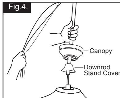
Step 4: Insert the motor wires through the downrod stand cover, canopy and downrod.
