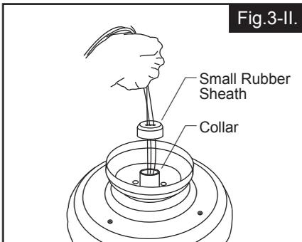
Step 3-II (for ceiling mount only): Thread the motor wires through the small rubber sheath. Attach the small rubber sheath fully cover onto the collar. Go to Fig.10 for the next step.
