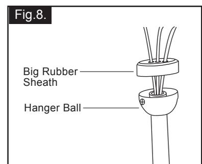
Step 8: Thread the motor wires through the rubber sheath, then fully cover it to the hanger ball.
