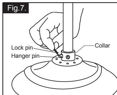
Step 7: Insert the hanger pin through the holes of the collar and downrod. Insert the lock pin through the hole near the end of the hanger pin until it snaps into its locked position. Finally, tighten two downrod screws on the collar.
