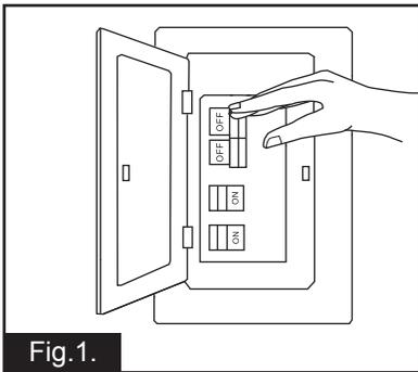
Step 1: Turn off the electric power at the main fuse or circuit breaker box.
