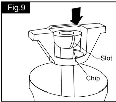
Step 9: Hang the fan on hanger bracket, and make sure the slot of hanger ball is snapped into the chip of hanger bracket exactly.
