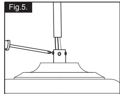
Step 5: Loosen the two downrod screws on the collar.
