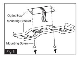
Tighten the mounting bracket to the outlet box with 2 mounting screws. (To reduce the risk of fire electric shock, or personal injury, mount to the outlet box marked "Acceptable for fan support" and use mounting screws provided with the outlet box.)
