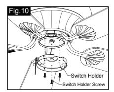
Secure the switch holder up to the bottom of the motor with switch holder screws.
