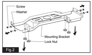
Remove the screws and washers from the mating holes on the mounting bracket. Remove the lock nuts from the mounting bracket.
