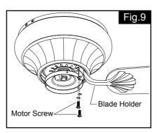
Attach blades to blade holders by using blade screws and washers.
