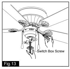
Secure the fan light onto the switch box using the switch box screws.
