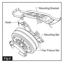
Attach one end of the mounting bar onto the hook of the mounting bracket. This will allow for hands-free wiring.
