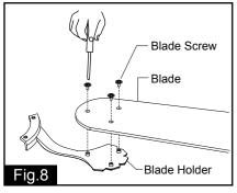
Tighten blades to blade holders by using blade screws and washers.
