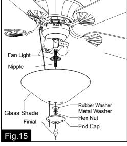
Install the glass shade, rubber washer and metal washer upward through the nipple and secure with hex nut. Then attach the end cap to the glass shade and secure it with finial. Take care to align the holes on the glass shade and the end cap, so that the pull chains pass through and move freely.
