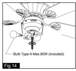
Install bulbs (included). See relamping label at socket area or packaging for maximum allowed wattage.
