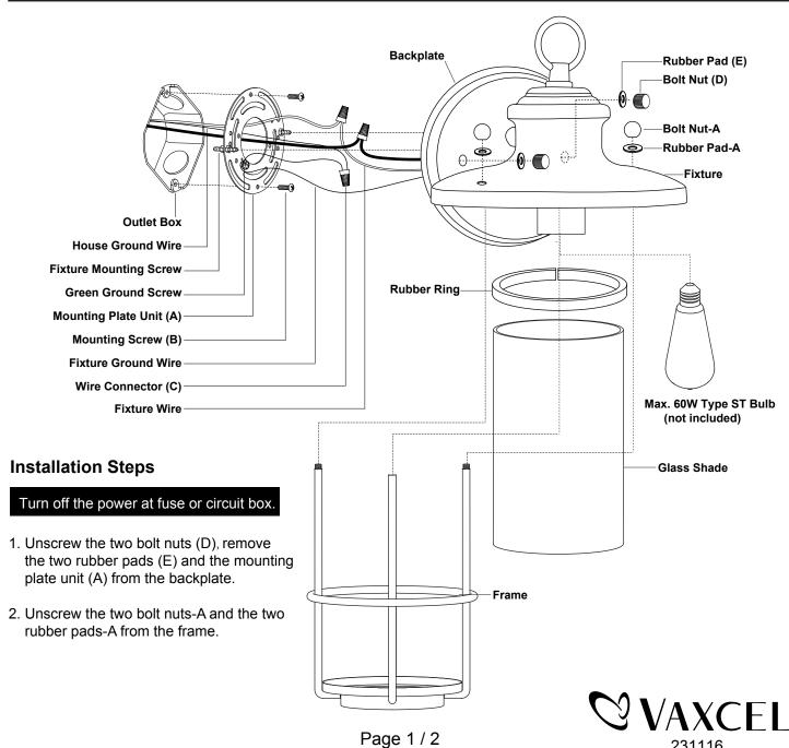
3. Attach the mounting plate unit (A) to the outlet box by using two mounting screws (B). Adjust the length of the preinstalled fixture mounting screws if necessary.
