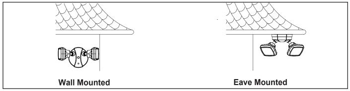
Light fixture should be mounted as shown above when installed (depending upon type of installation)
