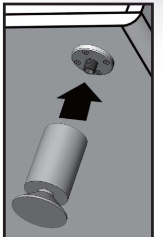
NOTE: Two Front Feet Only or Four Feet can be used with your cabinet. If installing optional feet, do so at this time.
