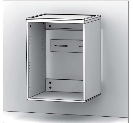
NOTE: For added stability, screw two additional screws into studs through the the top spanner (n) of the cabinet.
