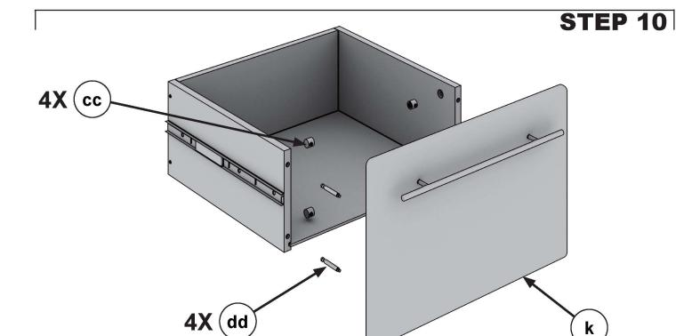
NOTE: Optional Handles should be installed in this step. UltiMATE GARAGE recommends 450mm pulls for GA-04P mounted horizontally.
