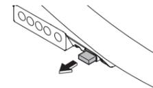
**4** Release your hand to return the water drain lever to its original position.
