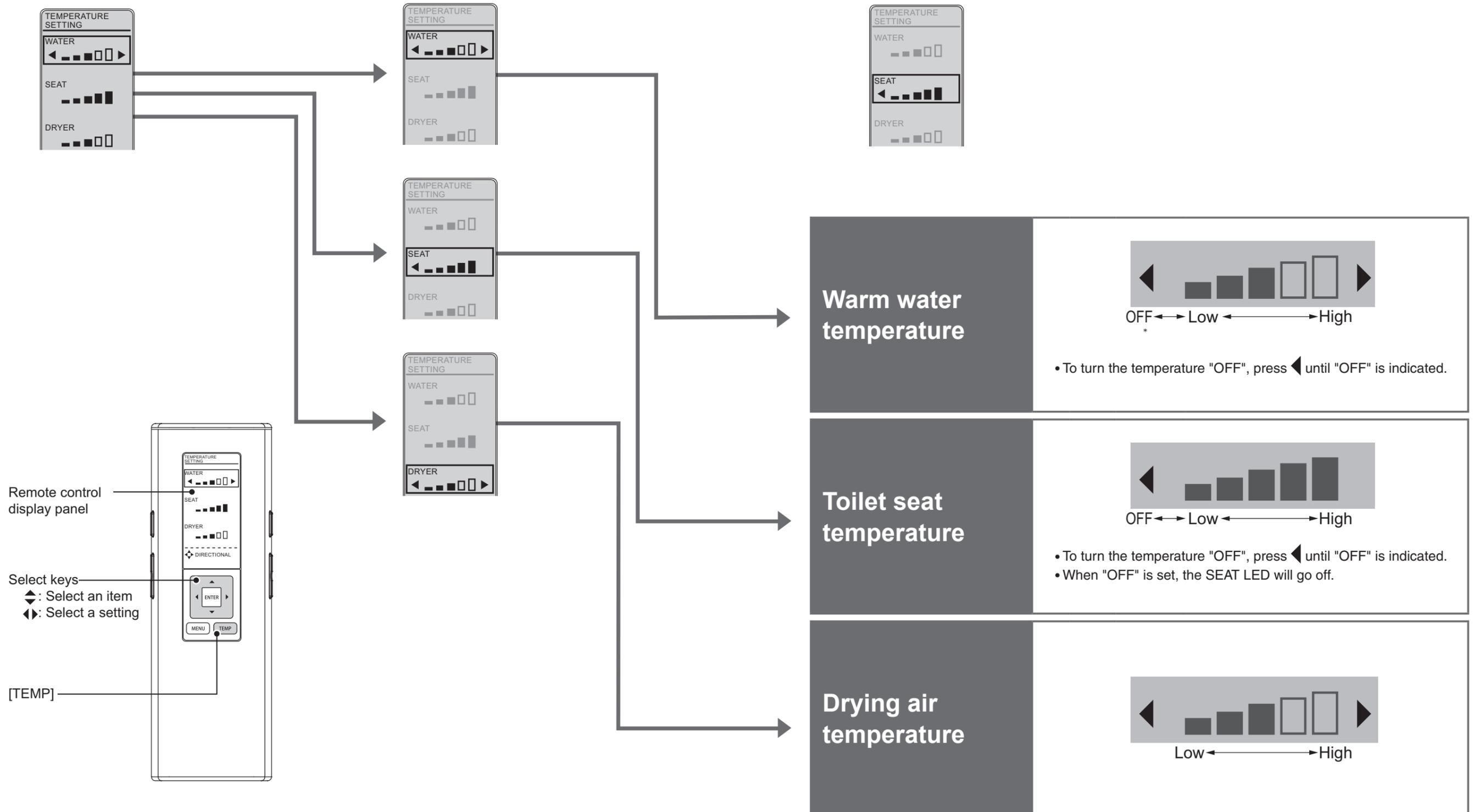
\* To prevent condensation, the warm water temperature does not drop below 20°C even when set to "OFF".
