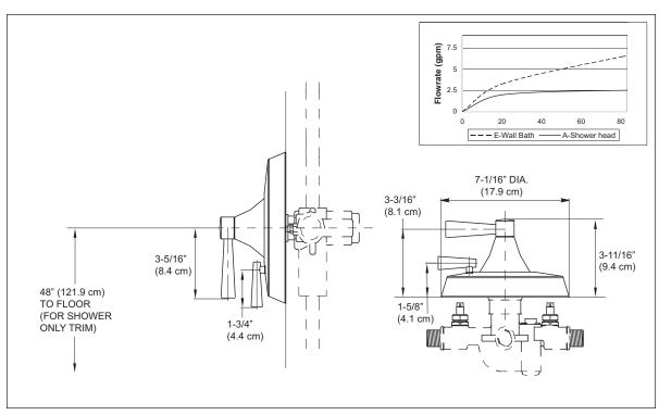
TS794PV - Nexus® Pressure Balance Valve Trim with Diverter
