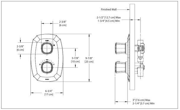
TS970CC - Guinevere™ Thermostatic Mixing Valve Trim with Single Volume Control
