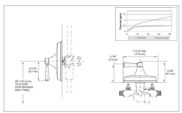
TS784P - Clayton® Pressure Balance Valve Trim without Diverter
