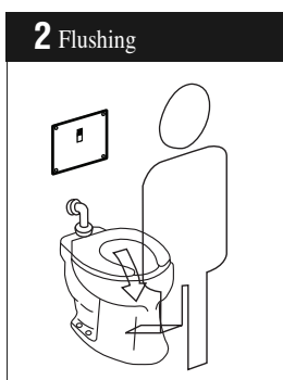
2 Flushing When the user stays in place longer than 6 seconds then moves away, the controller sends a signal to the operating unit to automatically trip the flush valve.
