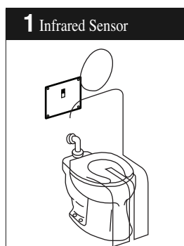
1 Infrared Sensor The infrared sensor detects a user sitting on the toilet seat.
