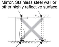
Infrared sensor of the automatic flush valve.
