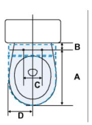
Note: Some styles of toilets may not allow the Washlet S300 to be installed due to certain contours near the tank and bowl area (see figures below). In the figure on the left side below, dimension D does not allow for enough open space to accommodate the minimum width of 9 inches.
