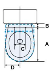
Note: Some styles of toilets may not allow the Washlet E200 to be installed due to certain contours near the tank and bowl area (see figures below). In the figure on the left side below, dimension D does not allow for enough open space to accommodate the minimum width of 9 inches.
