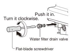
Tighten it securely using a flat-head screwdriver.
