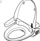
The seat switch is built in here.
