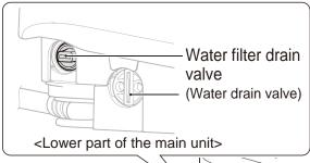
Remove the water filter drain valve.
