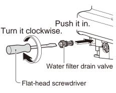
Tighten it securely using a flat-head screwdriver.
