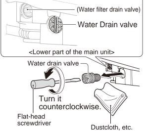
Loosen it by flat-head screwdriver.
