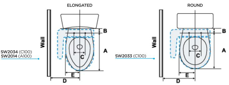
**Note:** Some styles of toilets may not allow the Washlet C100/A100 to be installed due to certain contours near the tank and bowl area (see figures below). In the figure on the left side below, dimension D does not allow enough open space to accommodate the minimum width of 11 inches.
