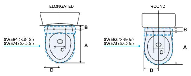
**Note:** Some styles of toilets may not allow the Washlet S300e/S350e to be installed due to certain contours near the tank and bowl area (see figures below). In the figure on the left side below, dimension D does not allow enough open space to accommodate the minimum width of 9 inches.
