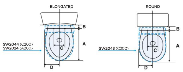
**Note:** Some styles of toilets may not allow the Washlet C200/A200 to be installed due to certain contours near the tank and bowl area (see figures below). In the figure on the left side below, dimension D does not allow enough open space to accommodate the minimum width of 9 inches.
