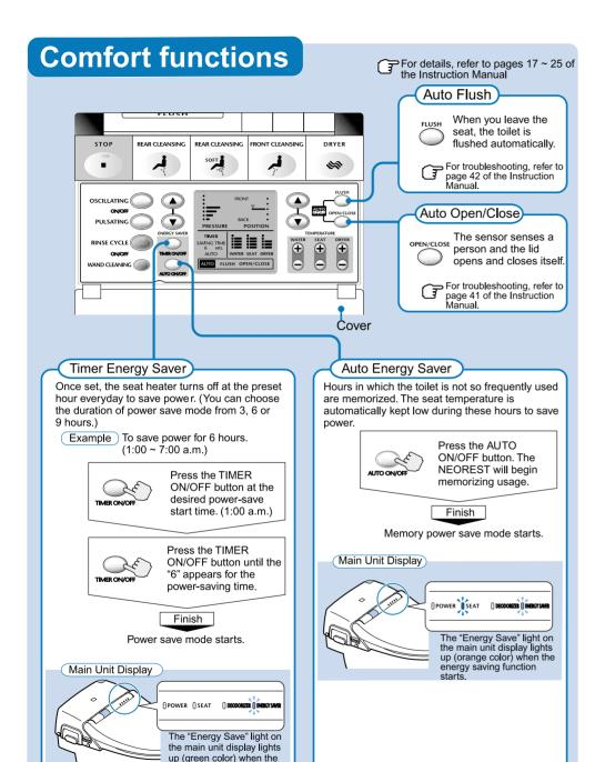
The timer energy saver and auto energy saver functions can be used simultaneously.
