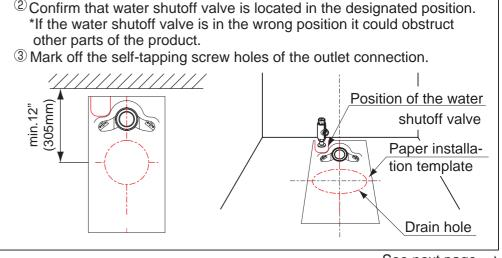
① Place paper installation template so that the base line of paper installation template and the center line of a toilet bowl match.
