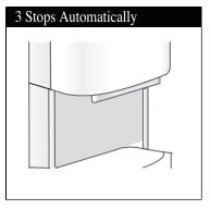
After hands are removed from the sensor's detection zone, or after sixty (60) seconds of continuous operation, the Hand Dryer automatically stops.
