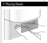
The infra red sensor detects a user's hands placed beneath the exhaust port.
