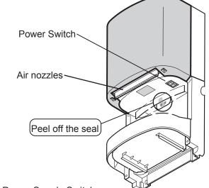
1. Check the main Power Supply Switch. • Turn on the main power supply switch on.
