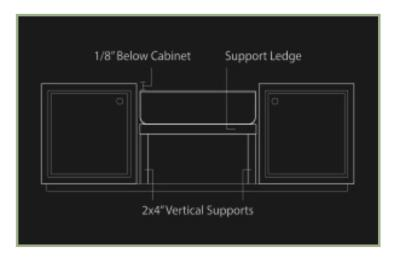
8. Cut the countertop with your template and install the countertop. Apply a bead of silicone sealant between the rim of the sink and the countertop to create a watertight seal.
