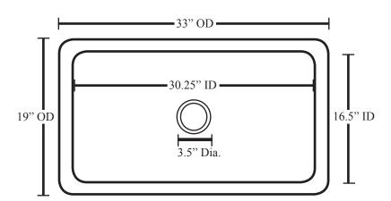
Your copper sink is handmade and therefore a work of art. Each sink is unique and can vary 1/4" in either direction. We highly recommend waiting to receive your sink before cutting your counter top.
