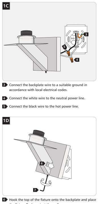
the fixture flush against the wall.
