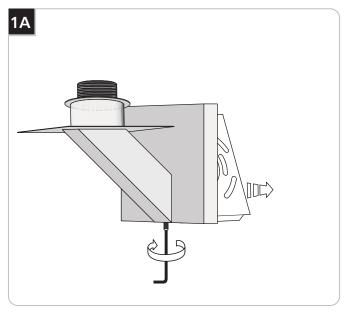
Back out the set screw at the bottom of the fixture and remove the backplate.
