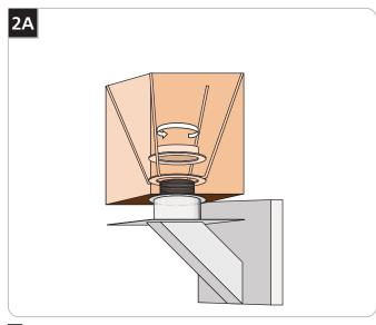
Place the shade support ring onto the socket and screw the retaining ring to the socket.
