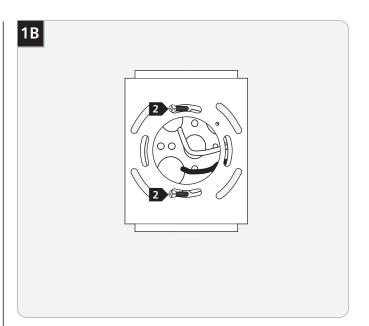
2 Screw the backplate to the electrical box.
