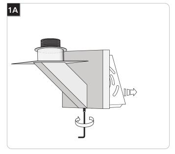
1 Back out the set screw at the bottom of the fixture and remove the backplate.
