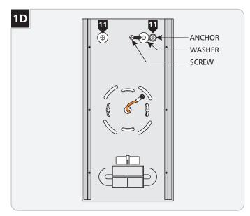
11 Slide a #8 screw through a washer, and screw it into an anchor to secure the fixture base to the wall. Repeat for the other anchor.
