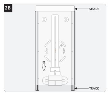
2 Gently slide the edges of the shade down the tracks in the fixture base until it rests against the end of the tracks.
