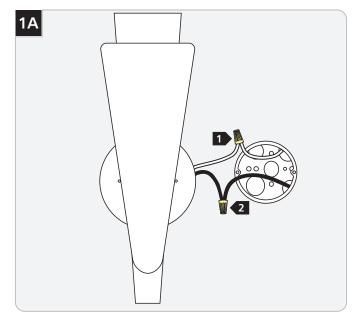
Connect the neutral power line wire to the white fixture wire with a wire nut.
