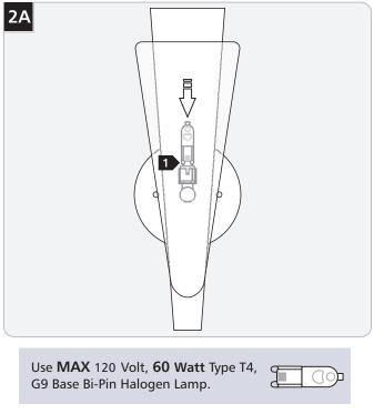
Push the lamp base into the socket.
