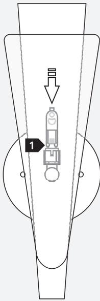
Use **MAX** 120 Volt, **60 Watt** Type T4, G9 Base Bi-Pin Halogen Lamp.
