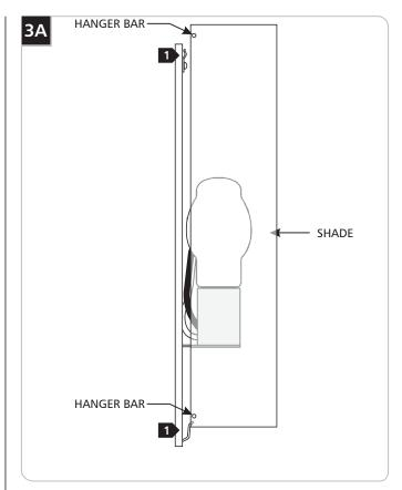
Slide the shade hanger bars onto the clips on the mounting plate.
