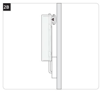
**NOTE:** Do not over tighten the thumb screw. Overtightening may break the glass and cause injury.
