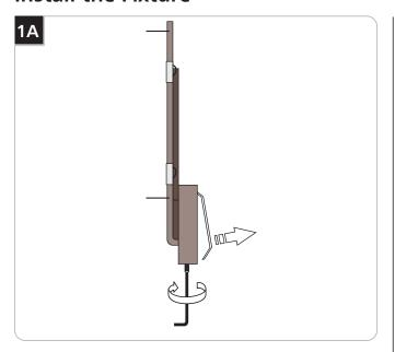
1 Back out the set screw at the bottom of the fixture and remove the backplate.
