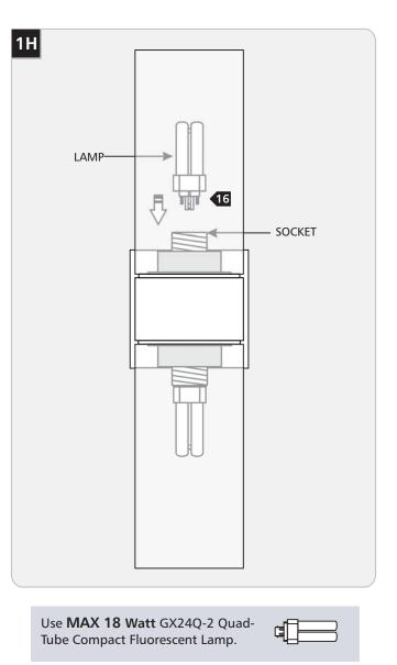
**16** Push the lamp pins completely into the socket holes, and repeat for the other side.
