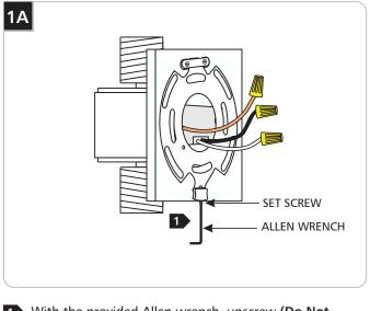
With the provided Allen wrench, unscrew (Do Not Remove) the set screw on the bottom of the fixture
