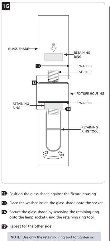
**NOTE:** Use only the retaining ring tool to tighten or loosen the retaining ring. Tightening or loosening the retaining ring by any other method can result in injury, or damage to the fixture.
