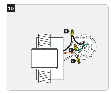
**6** Ground the fixture in accordance with local electrical codes.
