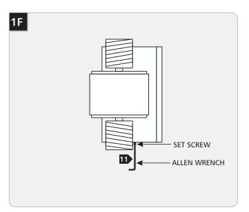
1 Line up the fixture on the wall and then secure it to the mounting plate by tightening the set screw at the base of the fixture.
