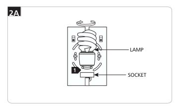
**CAUTION:** To reduce the risk of a burn or electric shock during relamping, disconnect power to the fixture.
