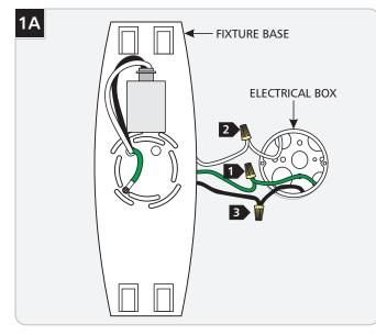
Connect the green ground wire to a suitable ground in accordance with local electrical codes.
