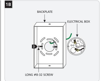
Mount the backplate to the electrical box with two long #8-32 screws.
