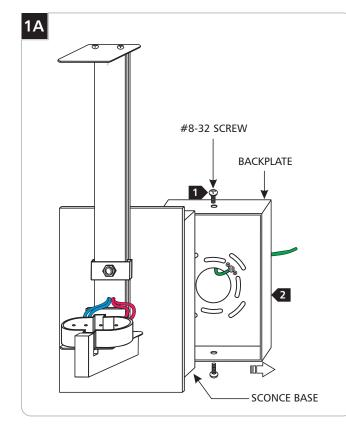
Remove the two #8-32 screws on the backplate with a Phillips head screwdriver.
