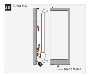
2 Line up the shade pegs on the sconce base with the holes in the shade frame and slide the shade into place.
