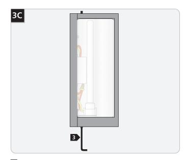
Tighten both #8-32 set screws using the provided 5/64" Allen wrench. Gently tug on the shade to verify that it is secured.
