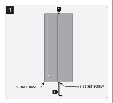
Back out both #8-32 set screws without removing them, using the provided 5/64" Allen wrench.
