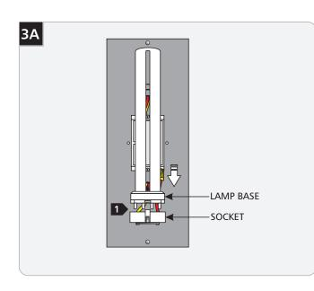
Push the lamp base firmly and completely into the socket.
