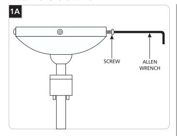
1 Separate the crossbar from the canopy by removing all four screws with the Allen wrench provided.
