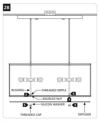
2 Adjust the nipples height by loosening the knurled nuts.
