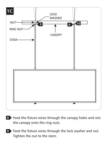
**10** Repeat the step 9 for the other fixture wires.
