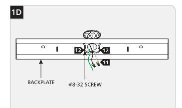
Feed the power line wires through the backplate center hole.
