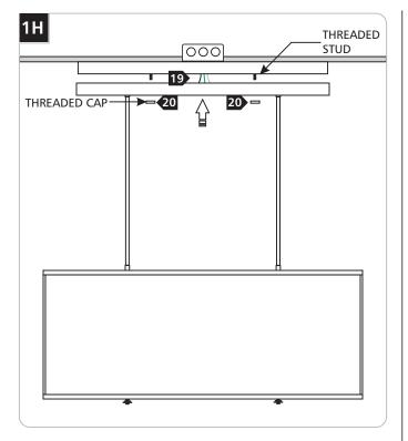
Place all wire and wire nut connections properly inside the canopy.
