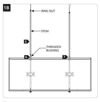
Feed the fixture wires through the stem (from the side without the ring nut).
