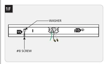
**15** Secure the backplate to the anchors with the #8 screws and washers.
