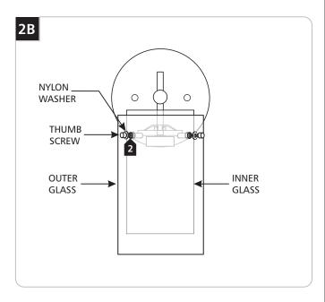
Line up the outer glass holes with the inner glass studs. Secure the outer glass to inner glass with provided three thumb screws and nylon washers.
