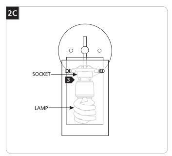
**CAUTION:** To reduce the risk of a burn or electric shock during relamping, disconnect the power to the fixture by turning the wall switch off.
