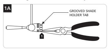
If the Soda accessory fits tight onto the fixture, then carefully bend the grooved shade holder tabs in slightly with the needlenose pliers. If it fits loose, then carefully bend the grooved shade holder tabs out slightly with the needlenose pliers.
