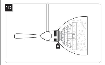
6 Hold the lamp against the glass with the thumb and push the lamp pins completely into the socket holes; simultaneously push the Soda accessory metal ring onto the grooved shade holder.
