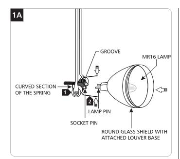
Use MAX 50 Watt MR16 Front Cover Halogen Lamp.
