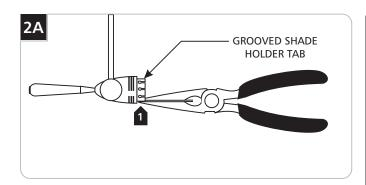
If the glass shield fits tight onto the fixture, then carefully bend the grooved shade holder tabs in slightly with the needlenose pliers. If it fits loose, then carefully bend the grooved shade holder tabs out slightly with the needlenose pliers.
