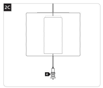
Use MAX 50 Watt Bi-Pin Halogen Lamp.
