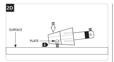
Tap the conical connector on a hard surface with the set screw facing down, so the plate inside drops into place.
